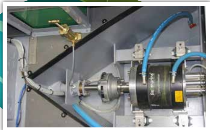
Electra community boat electric propulsion motor drive image courteous of Colecraft Engineering Ltd.
